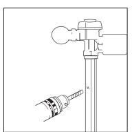
Use 6mm drill bit to drill a hole on urinal / WC pipe.
