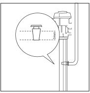
Insert the rubber nipple onto the 6mm hole. (Use pen knife to cut away 5mm lenght of nipple if installed on 16mm diameter urinal pipe).
