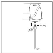
Insert plastic screw and 'O' ring into one end of pipe and metal screw into the other end.
