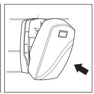
Replace cover by pushing inwards and use key to lock cover.
