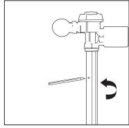
Mark the position of urinal / WC on the back of the pipe after loosening and twisting the pipe to the side.
