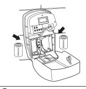
6 Insert 2'D' size batteries into battery compartment.
