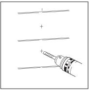
Drill 6mm diameter holes with approximately 6mm depth.
